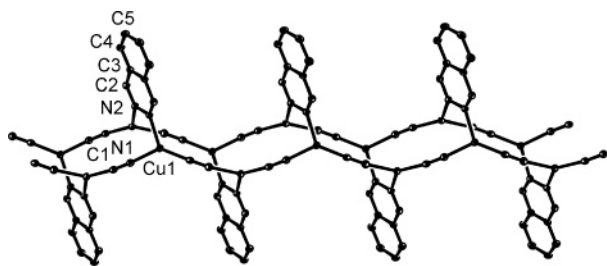
Figure 10. X-ray crystal structure of (\text{CuCN})_2(\text{Ptz}) , 12c . Hydrogen atoms omitted for clarity. Thermal ellipsoid view (50%).
